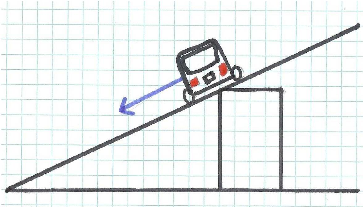
First I built a small car out of Fischer Technik. Then I went outside and placed one side of the board on the bucket, such that the board is tilted. Next I put the plastic table cloth on the board and sprayed water on it. Then I put a car on the board and made the board steeper. I then measured at what point the car would lose grip and slide down the wet tablecloth. In this experiment, a steeper board simulates a tighter turn.
