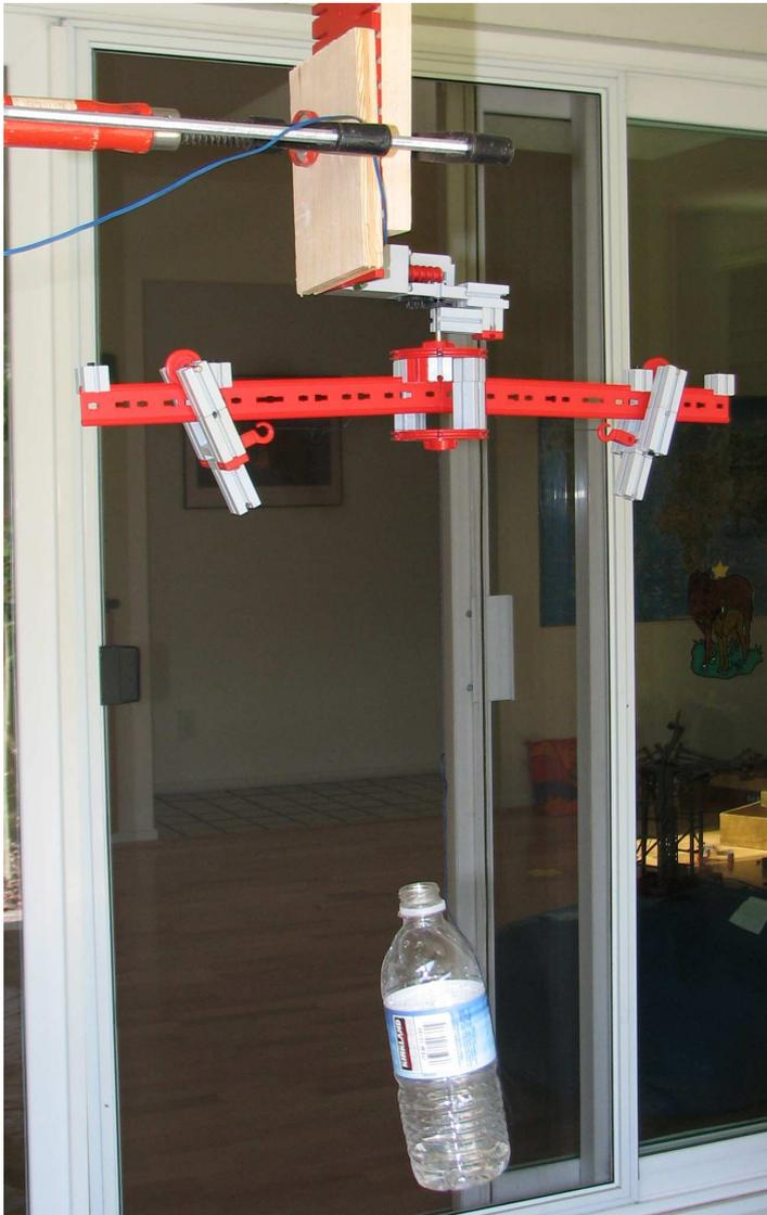
built two small carts that fit on the pole and put them on. Next I tied the thread to the carts. Then I connected the other side of the thread together and added a water bottle. After that I connected the motor to electricity and the pole started to spin. I then added or took away the water from the bottle until the carts went to the outside part of the pole. Next I measured the weight of the water bottle. After that I added weight to the carts and did the same process.
