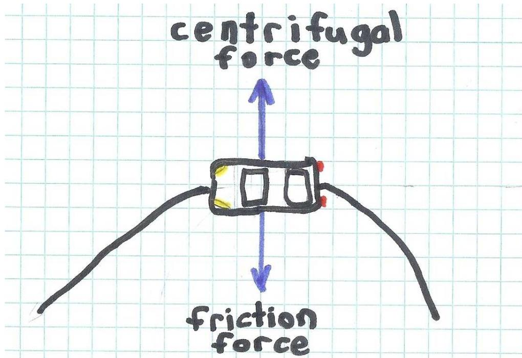
Skidding happens if the centrifugal force is larger than the friction force. The light car has a small centrifugal force and a small friction force. The heavy car has a large centrifugal force and a large friction force. Therefore it does not matter how heavy the car is.
